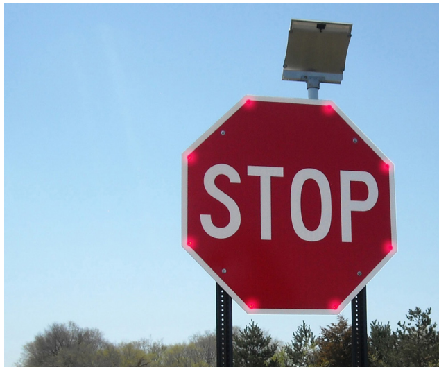
FIGURE 1: ENHANCED LED STOP SIGN
